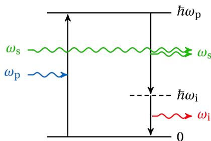
Figure 1: Optical Parametric Amplification
