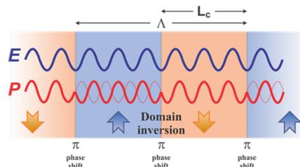
Figure 2: Quasi phase matching in a periodically poled nonlinear crystal.  $L_c$  is the coherence length,  $P$  is the induced light field, and  $E$  the pump field.
